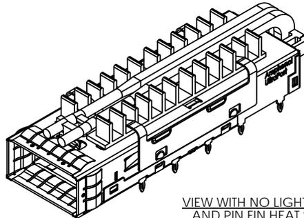
VIEW WITH NO LIGHT PIPE AND PIN FIN HEAT SINK (NO DUST COVER)
