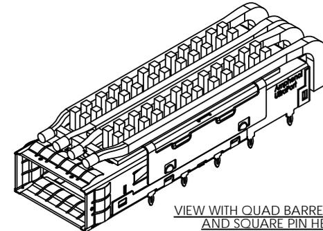
VIEW WITH QUAD BARREL LIGHT PIPE AND SQUARE PIN HEAT SINK (NO DUST COVER)
