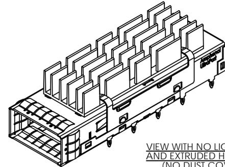
VIEW WITH NO LIGHT PIPE AND EXTRUDED HEAT SINK (NO DUST COVER)
