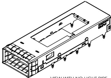
VIEW WITH NO LIGHT PIPE AND NO HEAT SINK (NO DUST COVER)
