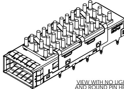
VIEW WITH NO LIGHT PIPE AND ROUND PIN HEAT SINK (NO DUST COVER)
